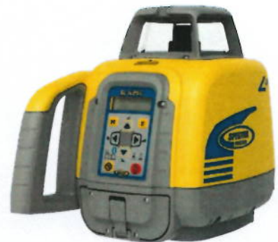
GL1425C features an enclosed lighthouse for superior ruggedness and environmental protection
