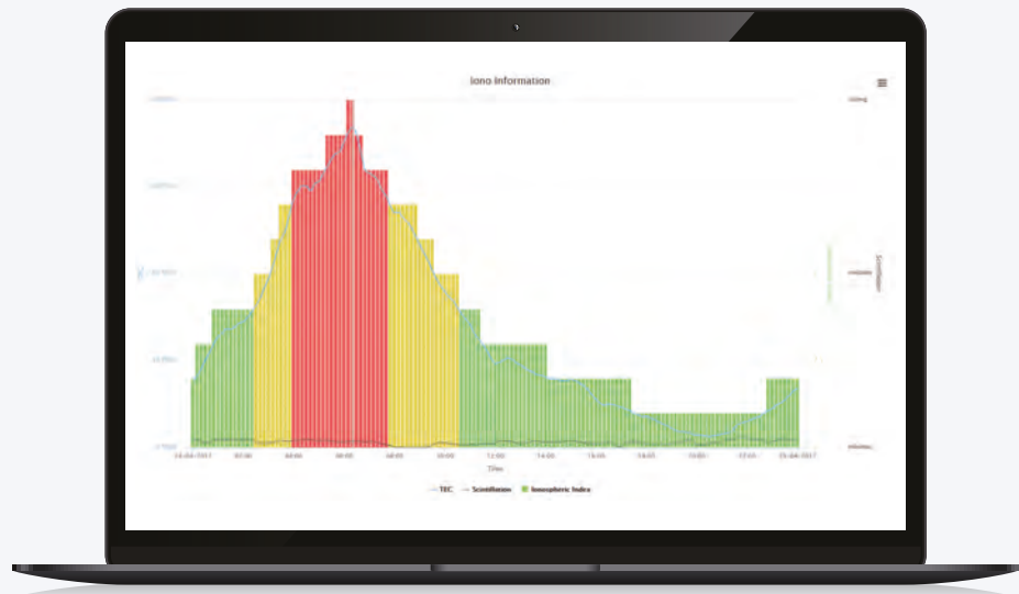
An ionospheric index value for a given location and time is also provided. This is a value on a scale of zero to 10 indicating ionospheric level derived from measured TEC and scintillation.
