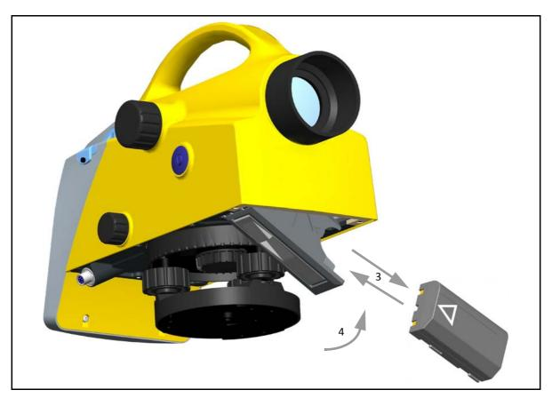
Figure 3.2 Inserting or removing the battery
