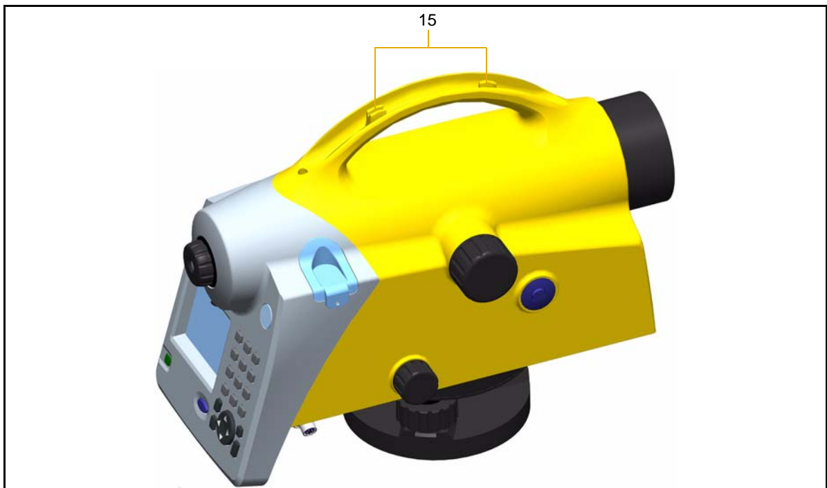
Figure 3.5 Instrument description, sight vane
